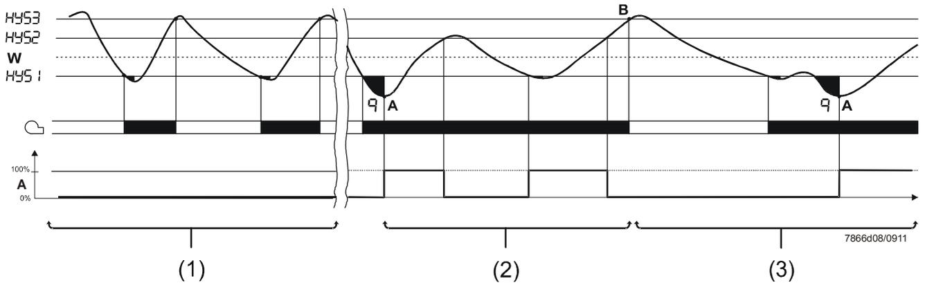
Figure 11: Control sequence of 2-stage burner, analog output
