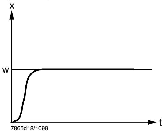
Figure 31: Optimum adjustment
