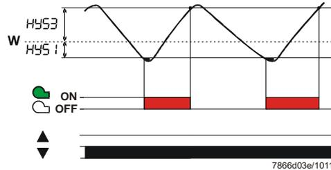
**Modulating and 2-stage operation:** Actual value lies between switch-on threshold HYS1 and switch-off threshold HYS3.
