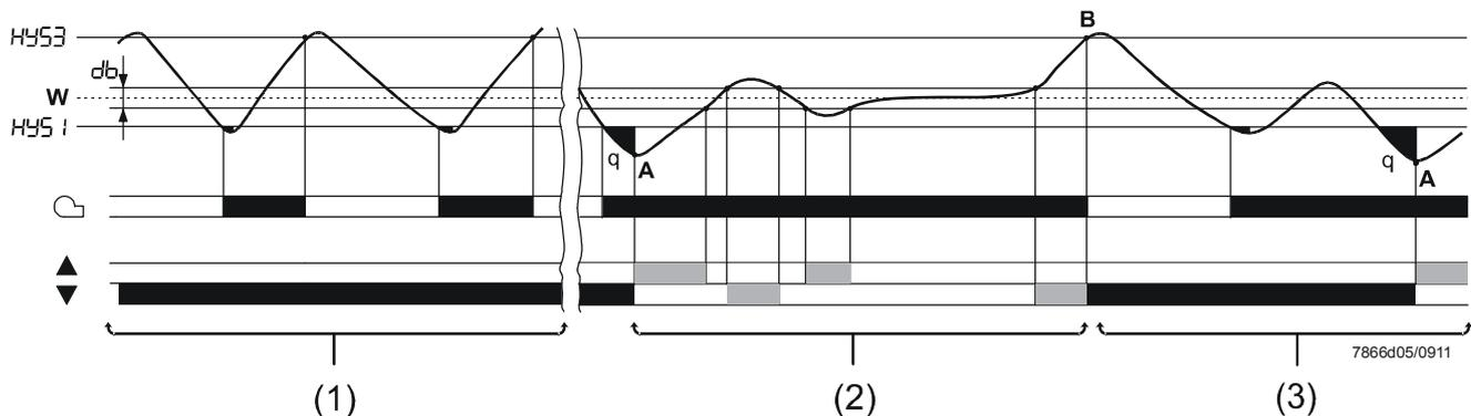
Figure 8: Control sequence of modulating burner, 3-position output
