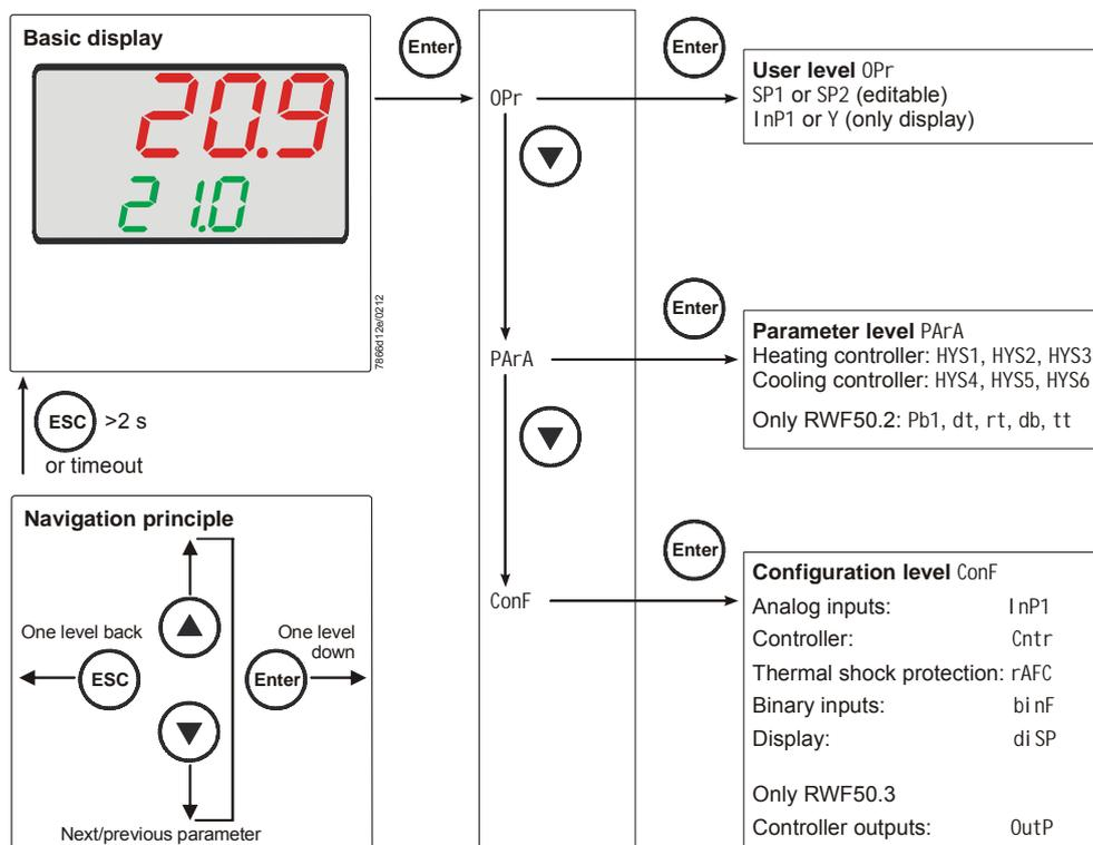
Figure 22: Parameterization
