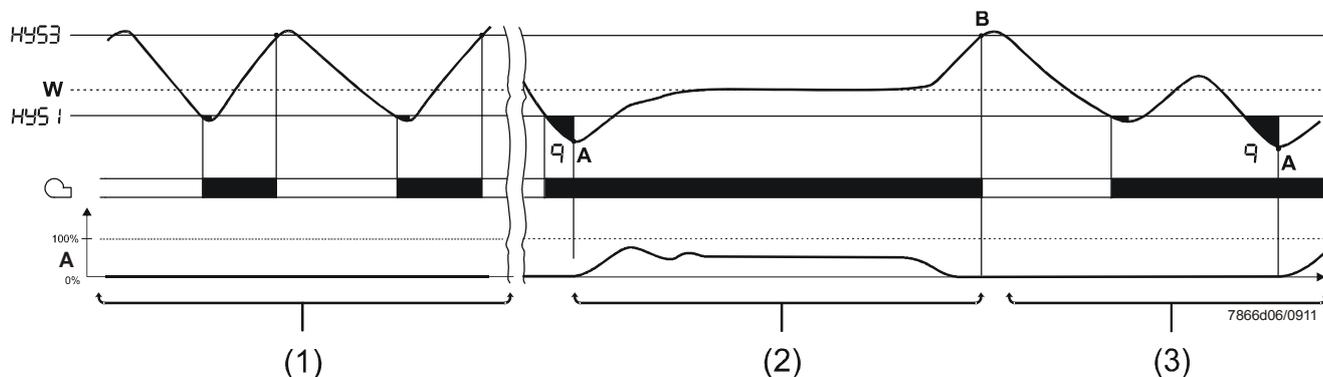
Figure 9: Control sequence of modulating burner, analog output
