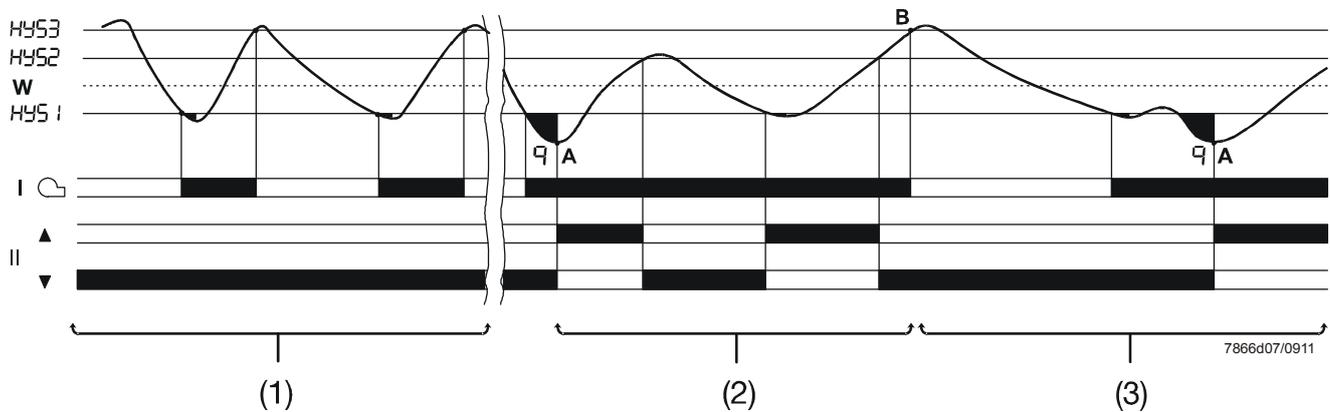
Figure 10: Control sequence of 2-stage burner, 3-position output
