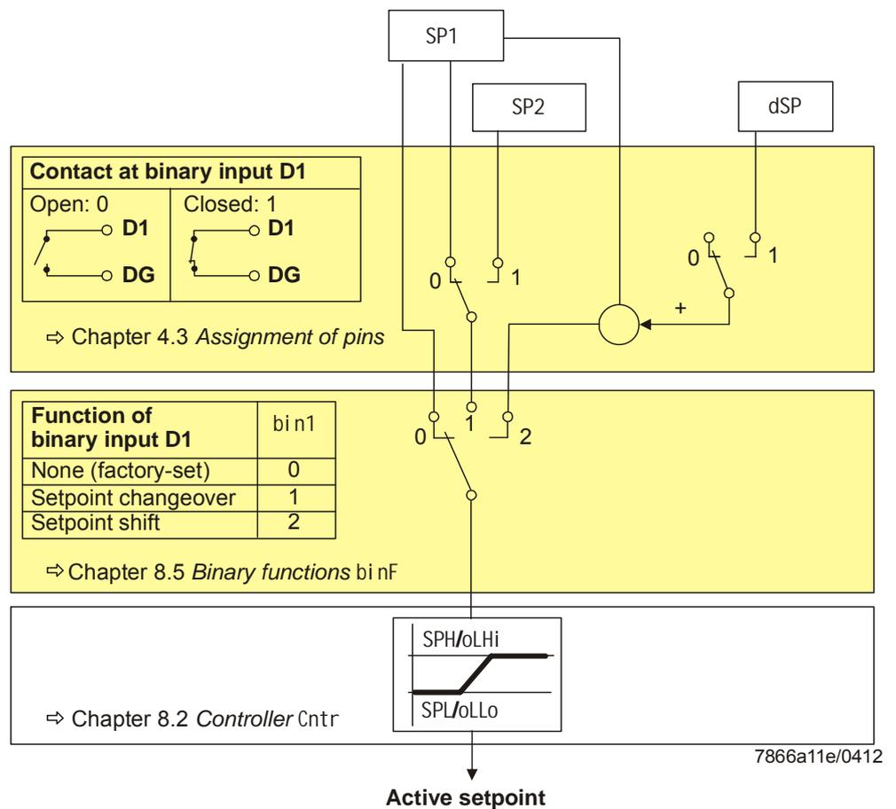
Figure 12: Setpoint changeover or setpoint shift
