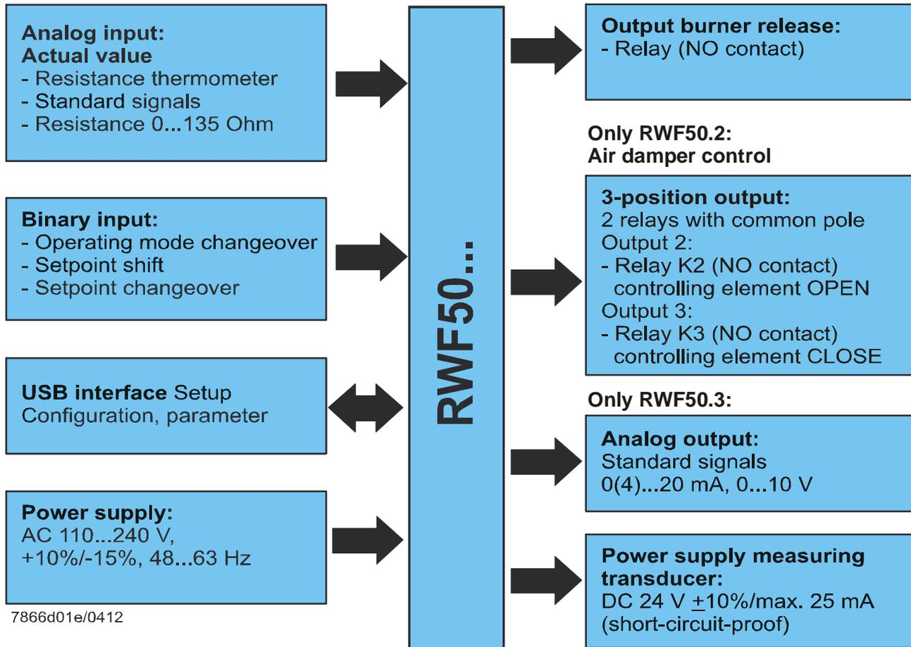
Figure 1: Block structure
