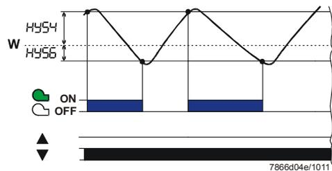
**Modulating and 2-stage operation:** Actual value lies between switch-on threshold HYS4 and switch-off threshold HYS6.
