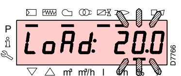
Press the key “F” for 1 second: “LoAd” is displayed and the load percentage flashes.
