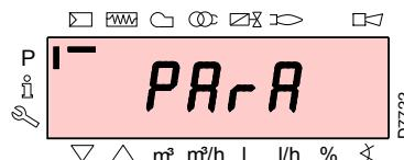
Select the group of parameters with keys "+" and "-", and confirm by pressing the "i/reset" key.
