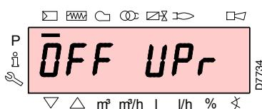
Check that the display of the Operator Panel shows request for heat and “OFF Upr”: this means it is necessary to set the modulation curve of the burner.
