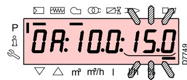
For the air servomotor, keep the key "A" pressed (the position in degrees flashes) and press the keys "+" or "-" to increase or decrease the value.
