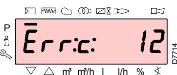
The display visualises alternately the error code (in the example alongside, c: 12) and the relative diagnostic (in the example d: 0).
