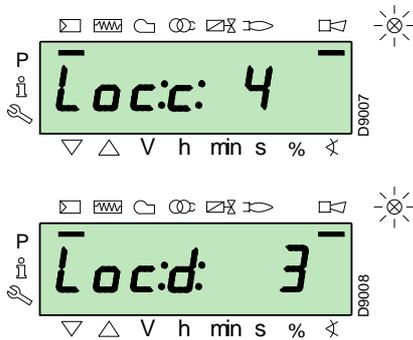
To reset, press the “i/reset” key for 1 s: the display will show “rESEt”. When the key is released, the lockout signal will disappear and the red indicator light will switch off. The control box is reset.
