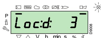
The display visualises alternately an error code and a diagnostic, which does not take the system into safety mode.
