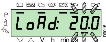
Releasing the “F” key, the standard visualisation appears, with the current load percentage flashing: this means that the burner is working in Manual mode (any outside adjustment is excluded and only the safety devices are active).
