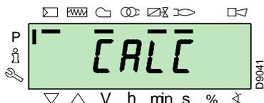
The control box will automatically calculate the points from “P8” to “P2”, distributing them in a straight line. These are theoretical and must be checked.
