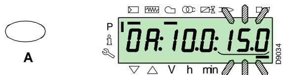
To adjust the speed of the inverter (expressed in % and that is **50 Hz = 100 %**), keep the buttons “F” and “A” simultaneously pressed, the percentage position blinks and press buttons “+” or “-” to increase or decrease the value.
