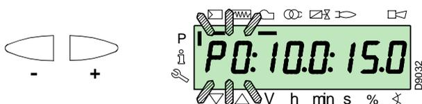
For the fuel servomotor, keep the key “F” pressed (the position in degrees flashes) and press the keys “+” or “-” to increase or decrease the value.
