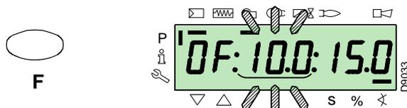
For the air servomotor, keep the key “A” pressed (the position in degrees flashes) and press the keys “+” or “-” to increase or decrease the value.
