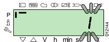
confirm with the button "i/reset" to activate the **restore** process.
