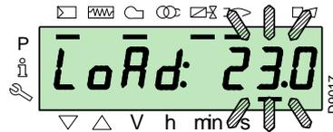
To exit manual mode, press the keys “+” and “-” (ESC) simultaneously for 3 seconds: the burner will work in Automatic mode and the output will depend on the thermostat/adjustment pressure switch (TR).
