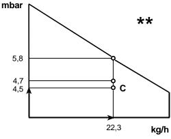
Delivery Q = 19 kg/h - Comb. chamber press. H1 = 5 mbar
