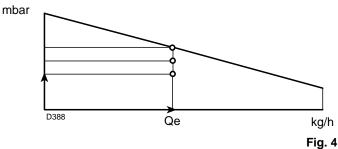
A reduction in delivery is accompanied by a reduction of the pressure in the combustion chamber:
