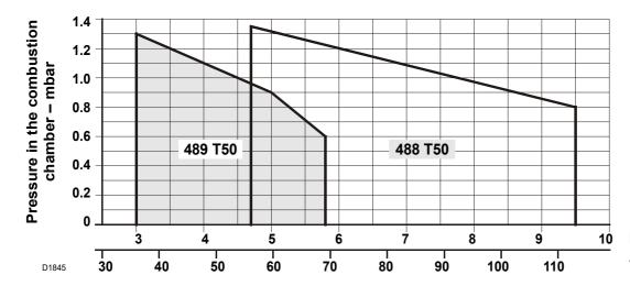
Fuel output - kg/h Thermal power - kW
