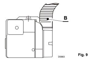
The combustion air supply is through a flexible or rigid pipe connected to the air intake.
