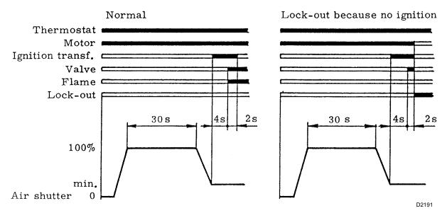
If during operation the flame shuts off, lock-out occurs within 1 sec.
