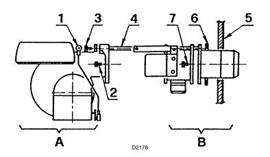
Separate the blast tube from the burner body by loosening the screws 7) and 3), fix the blast tube to the boiler front plate 5) using the gasket 6) provided.
