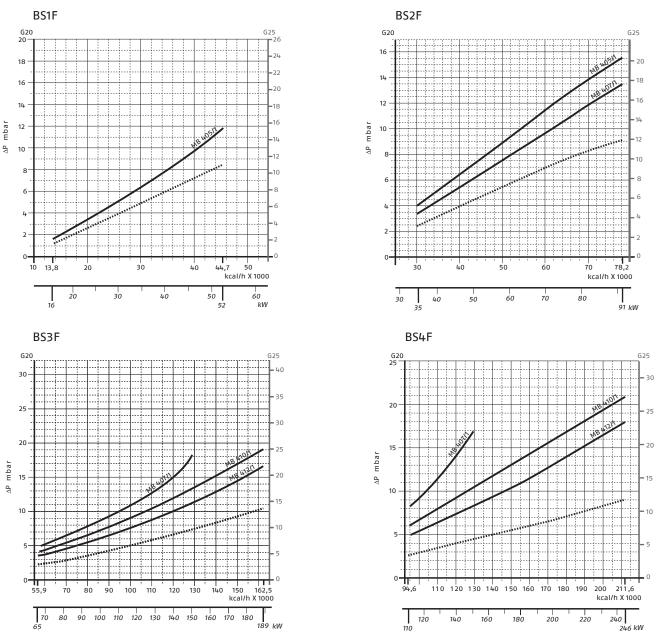
Please note: the diagrams indicate the minimum gas pressure drops of the burners equipped with the gas trains to be used (approved according to the EN 676 standard); in order to obtain the minimum pressure required at gas train inlet, combustion chamber counterpressure (expressed in mbar) must be added to this value. Combustion head + gas train
