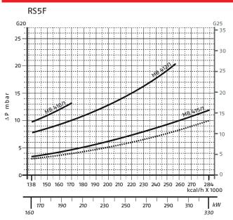
Please note: the diagrams indicate the minimum gas pressure drops of the burners equipped with the gas trains to be used (approved according to the EN 676 standard); in order to obtain the minimum pressure required at gas train inlet, combustion chamber counterpressure (expressed in mbar) must be added to this value. ----
