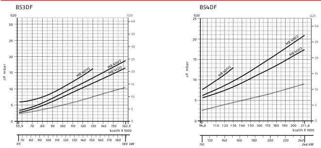
Please note: the diagrams indicate the minimum gas pressure drops of the burners equipped with the gas trains to be used (approved according to the EN 676 standard); in order to obtain the minimum pressure required at gas train inlet, combustion chamber counterpressure (expressed in mbar) must be added to this value. ——— Combustion head + gas train \_\_\_\_
