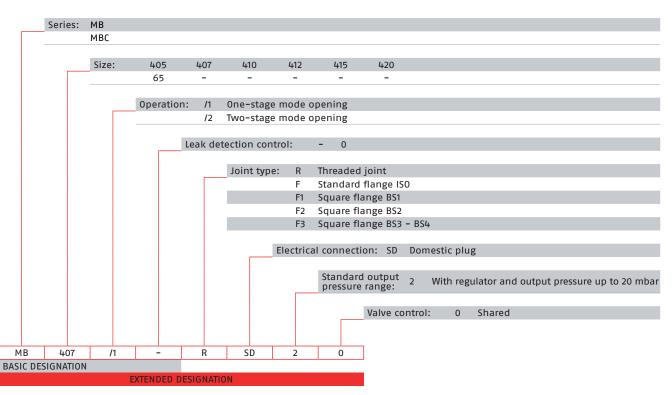
NOTE: in compliance with the European Standard EN 676, leak detection control devices are compulsory for burners with maximum outputs over 1200 kW.
