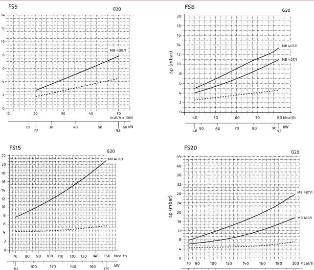
Please note: the diagrams indicate the minimum gas pressure drops of the burners equipped with the gas trains to be used (approved according to the EN 676 standard); in order to obtain the minimum pressure required at gas train inlet, combustion chamber counterpressure (expressed in mbar) must be added to this value. Combustion head + gas train Combustion head
