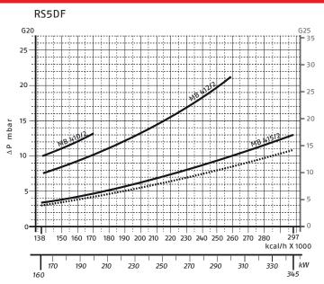
Please note: the diagrams indicate the minimum gas pressure drops of the burners equipped with the gas trains to be used (approved according to the EN 676 standard); in order to obtain the minimum pressure required at gas train inlet, combustion chamber counterpressure (expressed in mbar) must be added to this value.
