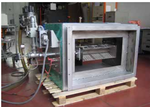
Thermal recuperative post-combustor (reduction of pollutants in the process air)
