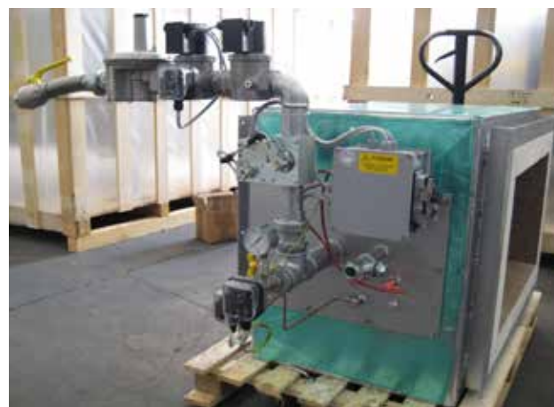
Thermal recuperative post-combustor (reduction of pollutants in the process air)
